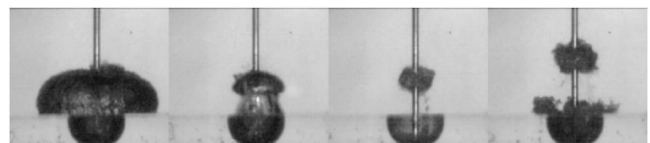
FIG. 13. Collapse, splitting, and rebound of an explosion bubble initiated at the bottom of a moderately sized hemispherical cavity.
